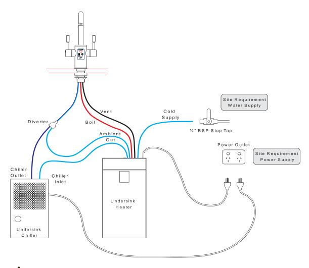
**WARNING**: The silicone piping from the Boiler/Chiller/Filtered tap to the Supatap must have a continuous fall to prevent the pipes from trapping water, twisting or folding. Failure to comply with this warning will cause the appliance to malfunction and void warranty. You may need to cut the piping to achieve the length required for a continuous fall.
