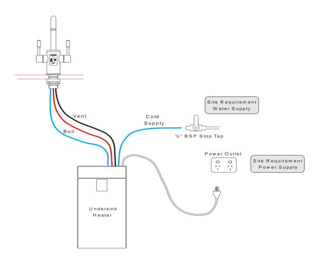
**WARNING**: The silicone piping from the Boiler/Chiller/Filtered tap to the appliance must have a continuous fall to prevent the pipes from trapping water, twisting or folding. Failure to comply with this warning will cause the appliance to malfunction and void warranty. You may need to cut the piping to achieve the length required for a continuous fall.
