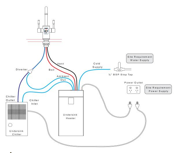
**WARNING**: The silicone piping from the Boiler/Chiller/Ambient tap to the Supatap must have a continuous fall to prevent the pipes from trapping water, twisting or folding. Failure to comply with this warning will cause the appliance to malfunction and void warranty. You may need to cut the silicone piping to achieve the length required for a continuous fall.
